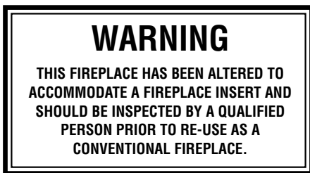
Figure 5 - Fireplace Warning Label
